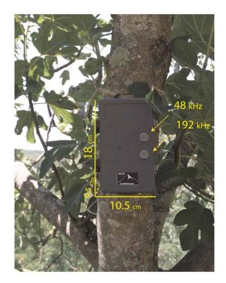
Figure 1. The Soundscape Explorer engineered by Lunilettronik (www.lunilettronik.it) is a terrestrial (SE[T]) and aquatic (SE[A]) automatic sound recording (Farina et al., 2016, 2018).
